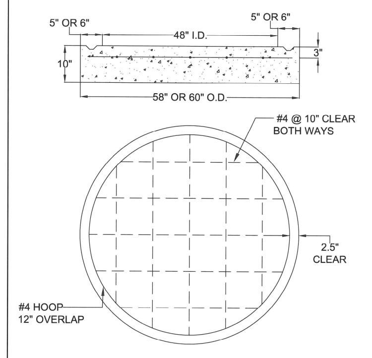
REINFORCEMENT MEETS OR EXCEEDS ASTM C-478 CONCRETE MIX DESIGN 4,000 P.S.I. @ 28 DAYS TYPE II/V PORTLAND CEMEMT
