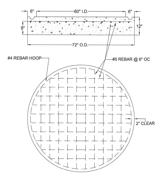
REINFORCEMENT MEETS OR EXCEEDS ASTM C-478 CONCRETE MIX DESIGN 4,000 P.S.I. @ 28 DAYS TYPE II/V PORTLAND CEMEMT
