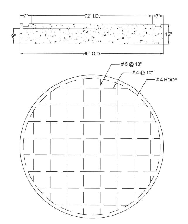
REINFORCEMENT MEETS OR EXCEEDS ASTM C-478 CONCRETE MIX DESIGN 4,000 P.S.I. @ 28 DAYS TYPE II/V PORTLAND CEMEMT
